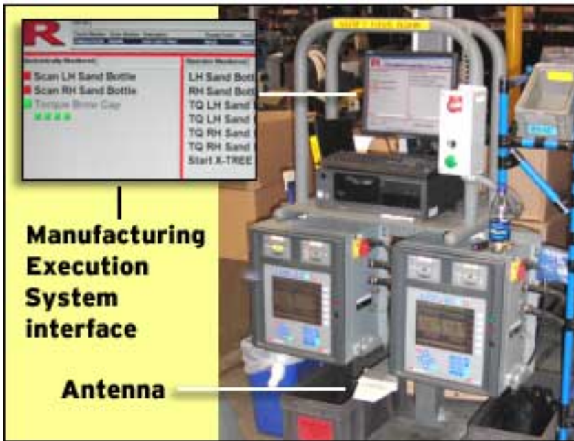
The RFID antenna located at each station is connected to the RFID transceiver card installed in the PC.
